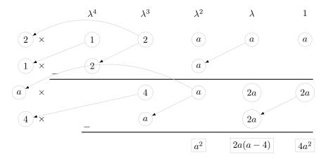
After the first step, we see that the system is stable if and only if a > 0 and the polynomial  $4\lambda^3 + a\lambda^2 + 2a\lambda + 2a$  is stable. After the second step, we see that the system is stable if and only if a > 0 and a - 4 > 0. This follows from the fact that a quadratic polynomial is stable if and only if all the coefficient have the same sign. Therefore, the system is stable if and only if a > 4.
